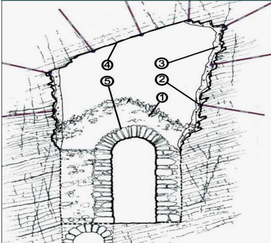
**Fig. 29:** Restoration measures at a large cave-in. Roman wall. **1:** Removal of debris, **2:** Stainless steel rock bolts, **3:** Concrete mantle, **4:** Short stainless steel nails and net, **5:** Arch strengthening
