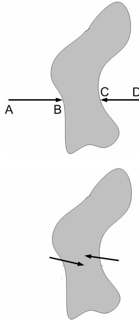
Fig. 4. (a) A sketch to show the two baselines necessary to guide the excavation of a tunnel from two portals through a rock mass indicated by shading. Accuracy in their alignment is critical. For the Samos tunnel the misalignment is of the order of  $0.5^\circ$  [4].
