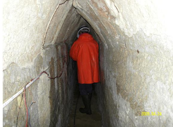
Figure 10. The measuring tape attached to the western wall of the Eupalinian Tunnel, 1.1 m above the floor, marks the tomographic transect that was carried out. The bunch of connecting cables is also shown. Electrodes were composed of bentonite mud mixed with salt (Tsokas *et al.*, 2006; Athanasidou *et al.* 2007b; Tsokas and Tsourlos, 2007; Tsourlos and Tsokas, 2011). This figure is available in colour online at [wileyonlinelibrary.com/journal/arp](http://wileyonlinelibrary.com/journal/arp)
